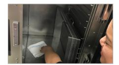
Remove left pan rail and lift steam collector to wipe dry and remove all moisture from the bottom of steamer.
